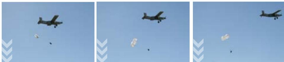
The maximum sink rate is measured during the last 30 meters, the paragliding wing is released, below or equal to 5,5 m/s under maximum load.
